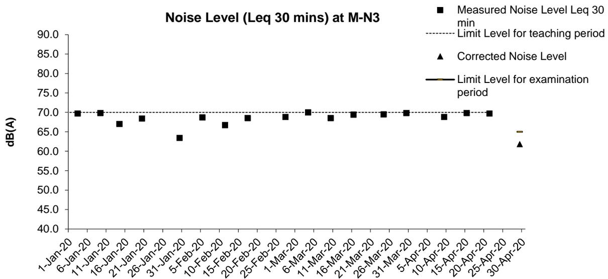
Remark: Corrected Noise Level was applied on 29 April 2020; Corrected Noise Level = Measured Noise Level - Baseline Noise Level (i.e. 67.7 dB(A))
